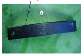
Remove the Grille (remove the 2 screws in the middle of the Grille)
