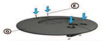
Align the two halves of the Base(G), make sure the wheel and axle are at right place. Insert bolts with washers ( $E \times 4 + C \times 4$ ).
