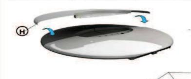
3 Attach each half of the metal cover. (Hx2) One half of the metal cover has a cut-out that should be placed over the rollers.
