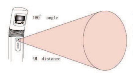
The PIR economy feature enables the outdoor heater to automatically shut down its heating function when not in use. The PIR sensor constantly monitors peoples movements up to a distance of 4 metres and if after 4 minutes it does not detect movement it will switch the heating off.
